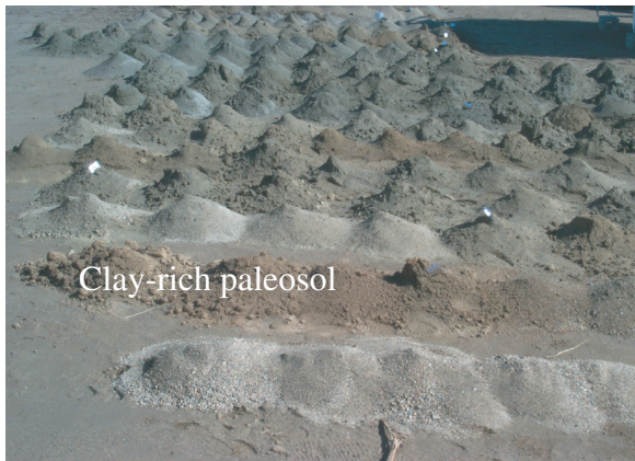
Figure 6. Heterogeneous alluvial deposits encountered during test drilling in the unsaturated zone underlying Oro Grande Wash near borehole VVWD, western Mojave Desert, California. Each pile represents the cuttings from a 0.3-m interval. Figure 1 shows the site location.
