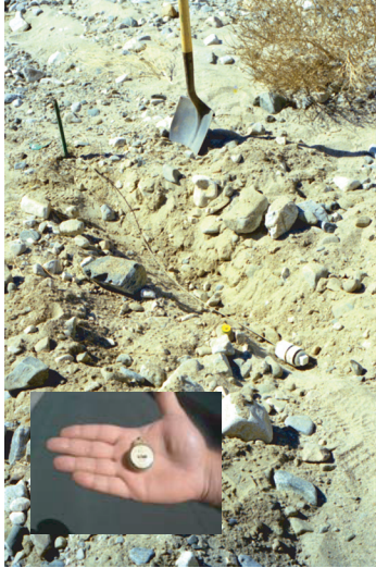
Figure 8. Streambed temperature site along Sheep Creek Wash near borehole USCW, western Mojave Desert, southern California. Inset shows close-up of temperature sensor. Figure 1 shows the site location.
