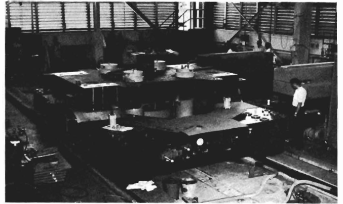
The undercarriage and bottom plate of the magnet. The bottom plate can be raised and lowered by four hydraulically synchronized lifting jacks. The whole carriage can slide on the rails which are lubricated by special material called Lubrite.
