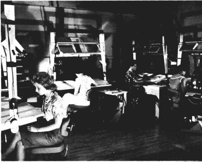
Scanning machines which project the picture by means of a lens and mirror onto a scanning table are used to find events of interest.
