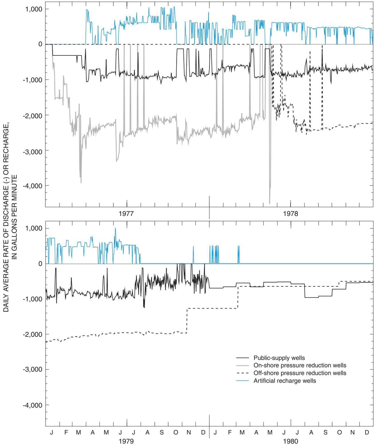
**Figure 9.** Daily average rates of discharge (-) from or recharge to wells on SUBASE Bangor, Kitsap County, Washington, 1977-80.
