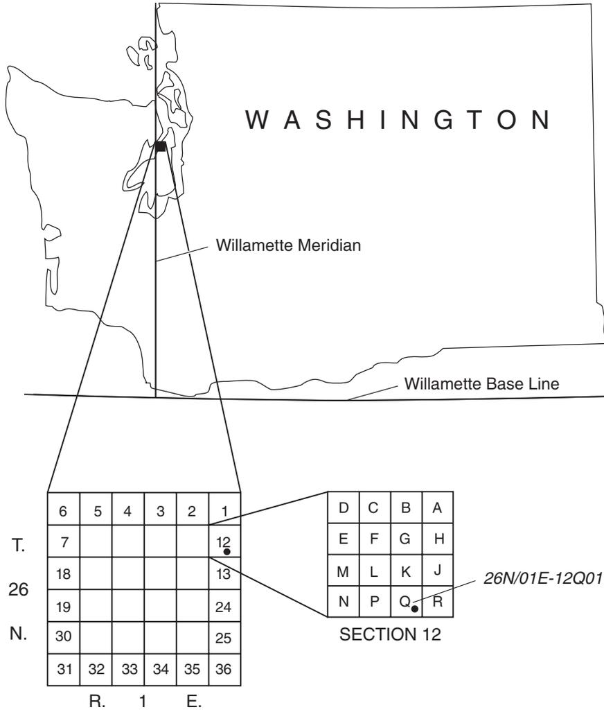
**Figure 3.** Well-numbering system used in Washington.
