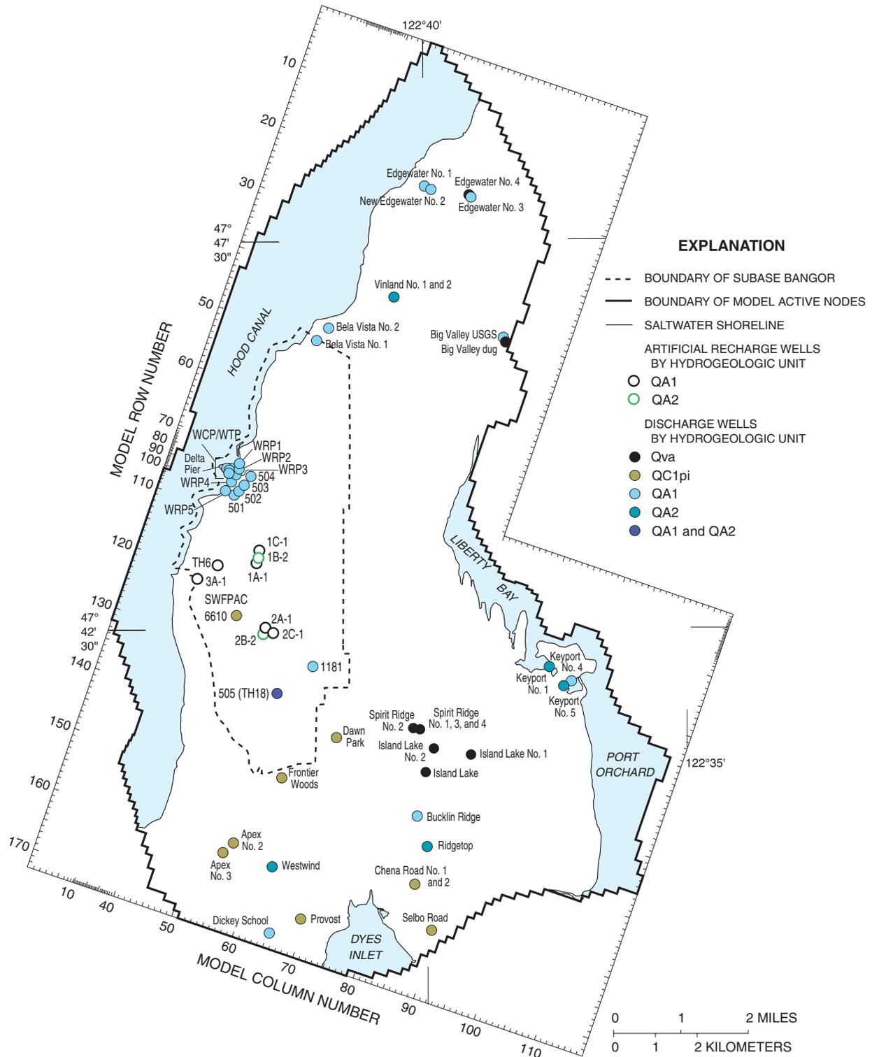
**Figure 8.** Locations of artificial recharge and discharge wells by hydrogeologic unit on SUBASE Bangor, Kitsap County, Washington.
