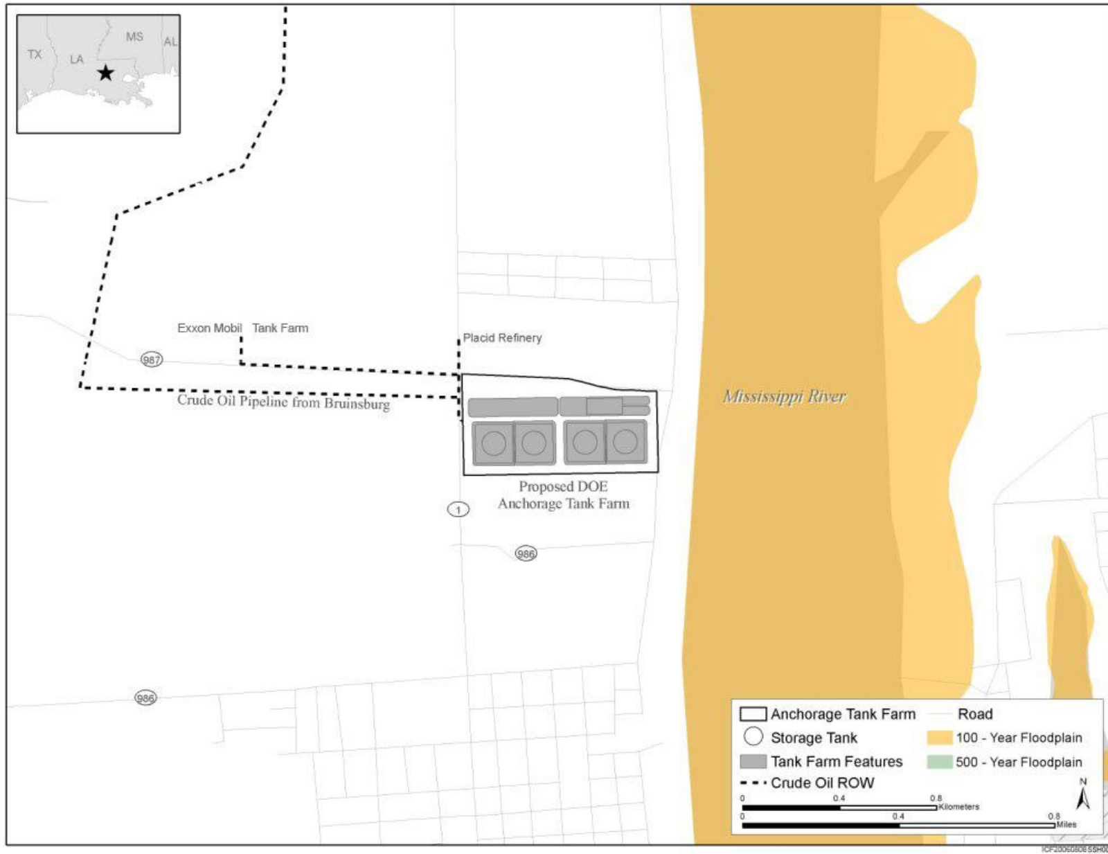
Figure B.6.1-3: Floodplain Map for Anchorage Terminal
