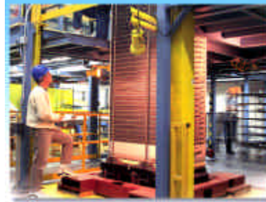
Cells stacked together for desired power
