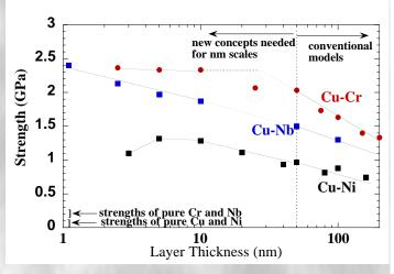
Strength (estimated as hardness divided by 3) vs.the layer thickness of several Cu-based multilayers. Note the significant increase in strength as compared to strengths of pure metals (estimated at  $10~\mu m$  grain size).
