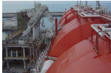
LNG is transferred from storage tanks (like these in Qatar) to the carrier ship via specially constructed loading systems.
