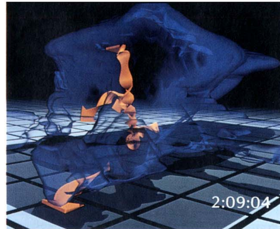
Tracer ribbons illustrate the development of streamwise vorticity during a 20-minute period. The relative magnitude of the vorticity is largest in the lower part of the storm, where the ribbon is most tightly coiled.
