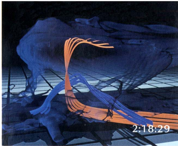
Orange ribbons represent tracers that rise through the depth of the storm in the updraft and blue ribbons represent tracers that eventually fall to the ground in the downdraft in this image tracing particle paths from approximately 75 minutes after the start of the simulation to 2 hours and 18 minutes after.
