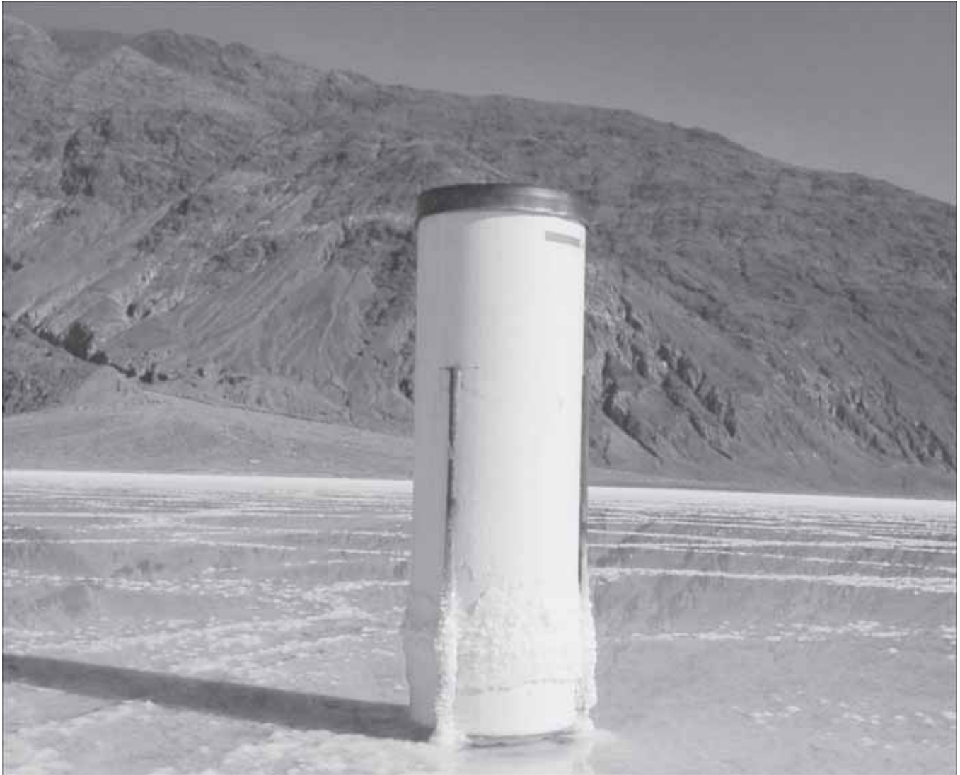
Figure 14. Salt-crystal deposits on a rain gage following the evaporation of surface flooding near the salt-encrusted playa micrometeorological data-collection site, Death Valley, California, April 2001.
