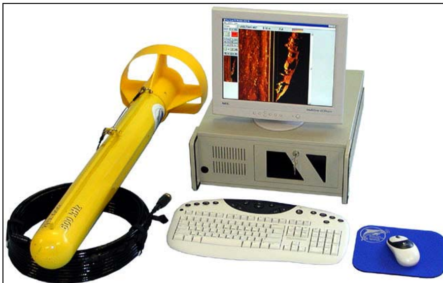
Figure 5-5. Marine Sonic Technology sidescan sonar system.
