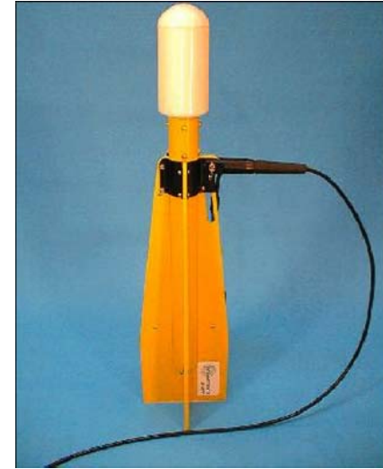
Figure 6.2 The G-877 proton precession marine magnetometer used in Task 3.
