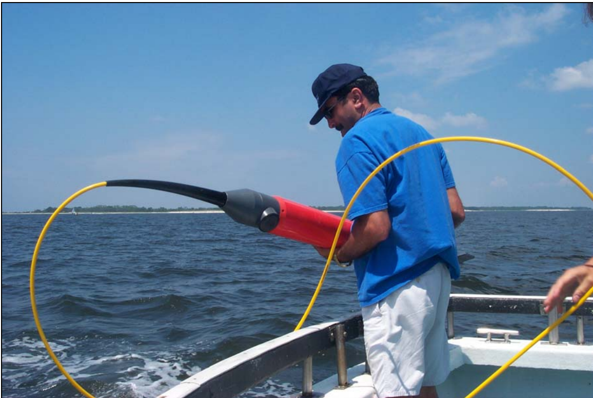
Figure 6-22. The Marine Magnetics SeaSPY magnetometer being deployed. Note the cylindrical altimeter sensor near the nose of the towfish.
