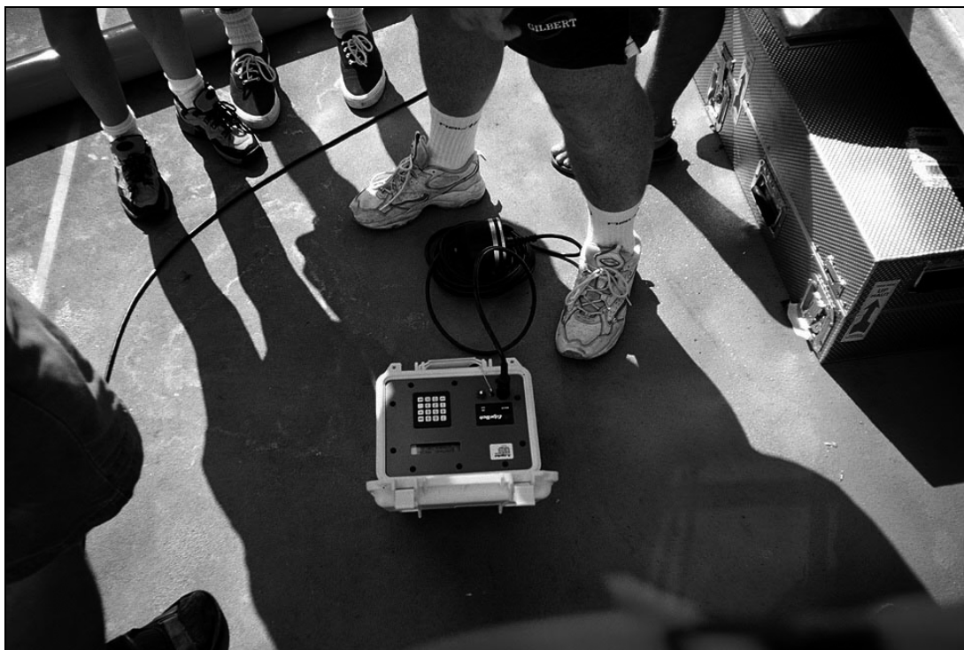
Figure 6-18. EdgeTech AMD200 Deck Unit Command Transmitter used to transmit a unique code to the CART.
