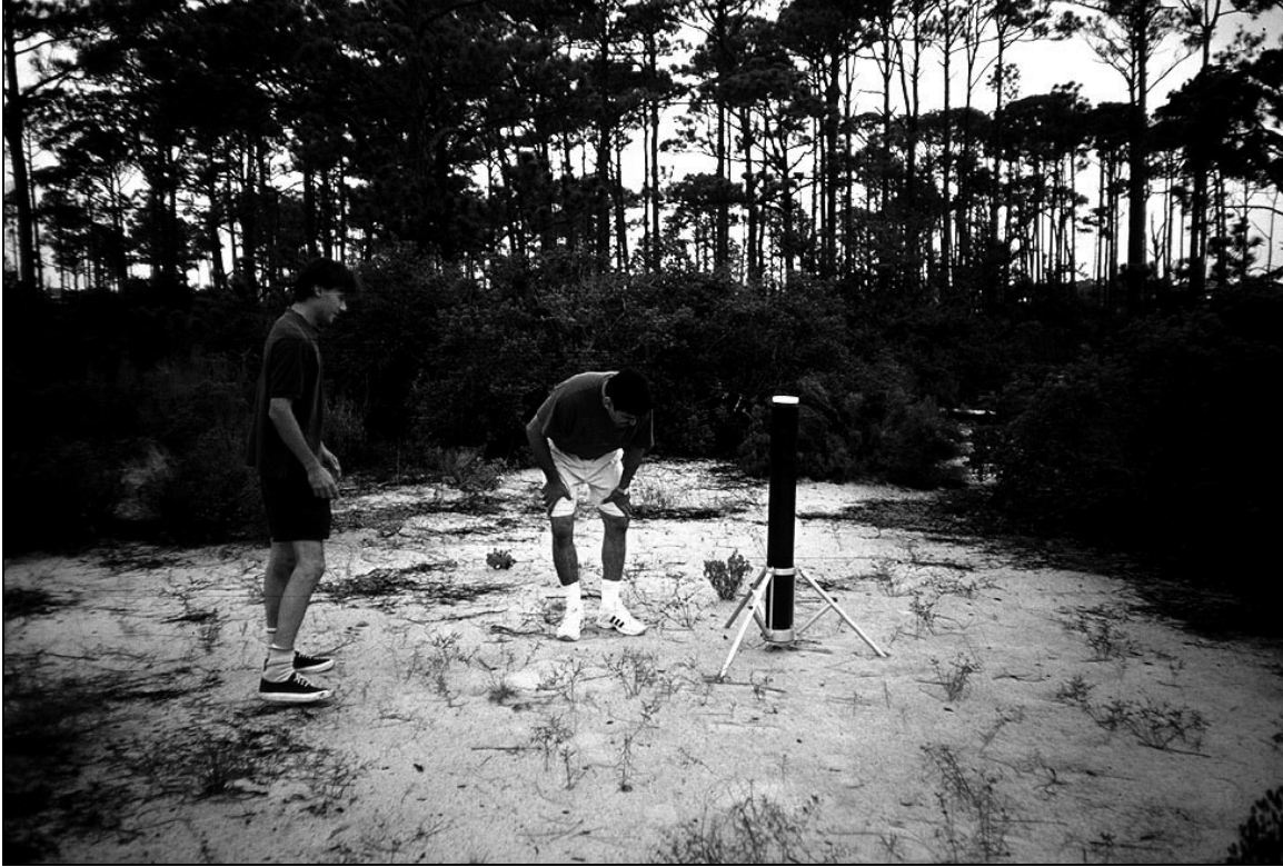
Figure 6-12. Marine Magnetics Sentinel base station being readied to collect data in Perdido Key, Florida.
