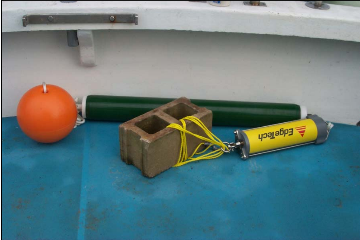
Figure 6-16. The Marine Magnetics Sentinel underwater base station prior to daily deployment.
