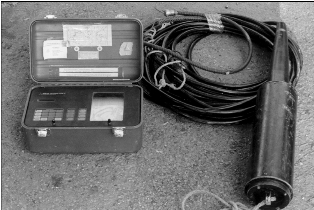
Figure 5-7. Geometrics Model G-866 marine magnetometer console and towfish.
