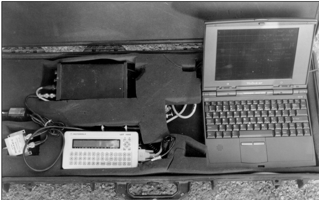
Figure 5-4. Differential global positioning system (DGPS) used for the project.
