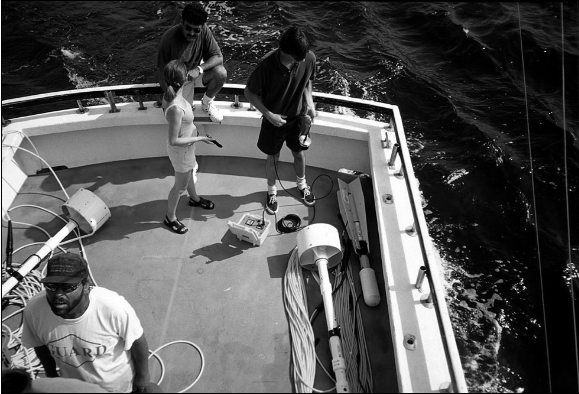
Figure 6-19. AMD200 transponder ready to place in the water.
