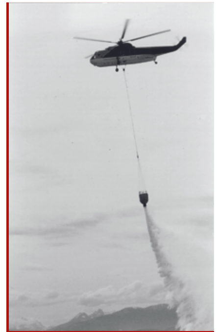
Figure 10—The hazards of helicopter operations include long cables that can tangle in trees, snags, or powerlines.
