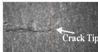
b) Internally Damaged Condition at ~ 30 kilocycles
