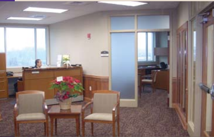
Textured glass panels are used in the NMC to fill interior spaces with natural light.
