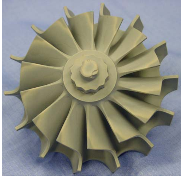
Figure 10. Photo of NT154 silicon nitride microturbine rotor manufactured by Saint-Gobain.
