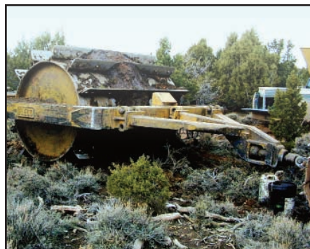
Figure 1. A roller chopper is effective in knocking down brush and trees and chopping up the slash.
