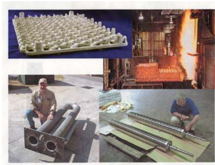
Figure 2. Nickel-Aluminide alloys in action: forms (top left) for automobile engine part casting (top right); heat exchanger (bottom left); rolling-mill rollers for steel-sheet manufacture (bottom right).
