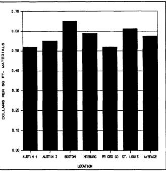
Figure 6. Installation Materials, Dollars Per Square Foot.
