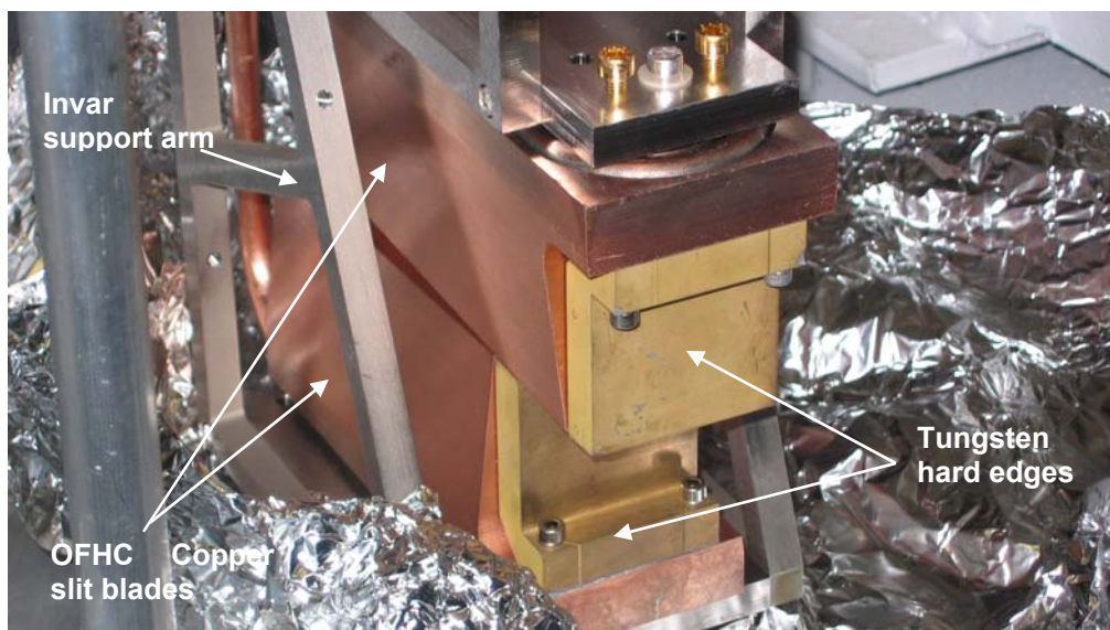
Figure 2.9. High-heat-load slits as used on HXMA ID06 beamline at CLS (designed to operate with >4kW power load).
