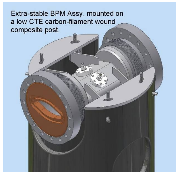
Figure 4.9.9 Design of the high-stability BPM support.
