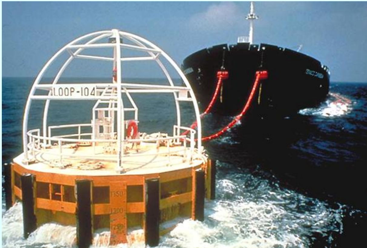
Offloading via Single-point Mooring Buoy
