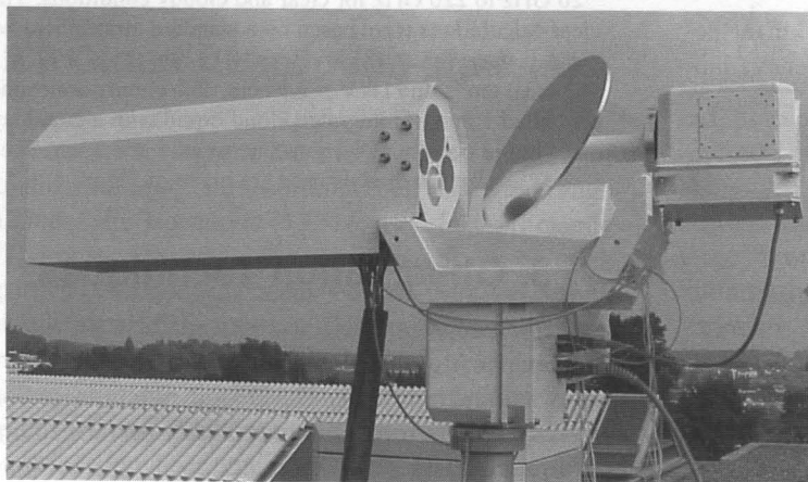
Figure 3. The ASMUWARA in operation in Bern. The openings of the four horns appear as grey disks at the left of the rotatable mirror, while the IR radiometer looks through the white cylinder below the largest horn.
