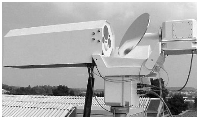
Figure 3. ASMUWARA in operation the IAP in Bern, Switzerland. The openings of the 4 horns appear as grey disks at the left of the rotatable mirror, while the IR radiometer looks through the white cylinder below the largest horn.
