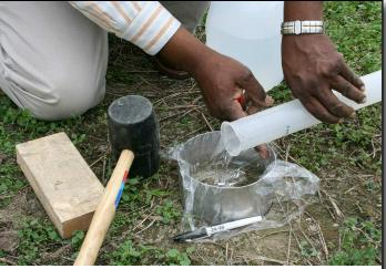
A one inch layer of water is added to a six inch diameter ring to measure infiltration rate.
