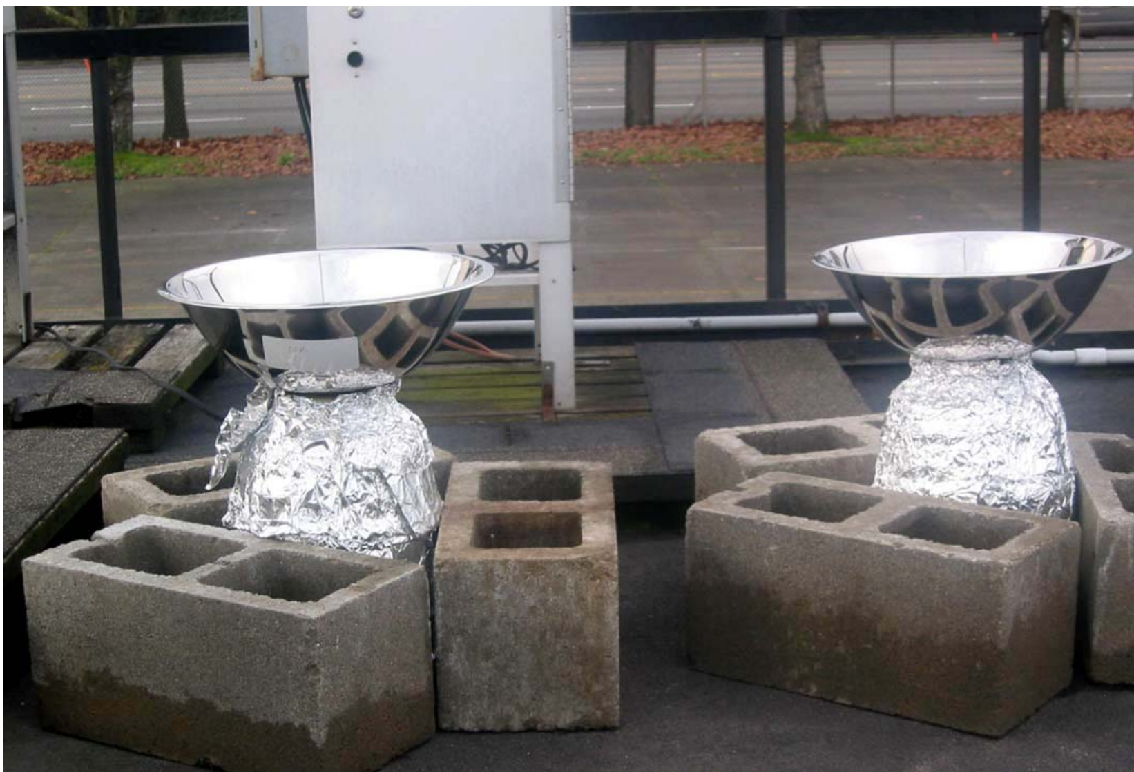
Figure 7. Wet/dry atmospheric deposition sampler
