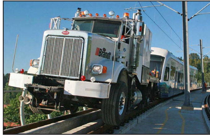
A light rail car gets an assist from the “Brandt,” a tow truck that can run on rails as well as the street.
