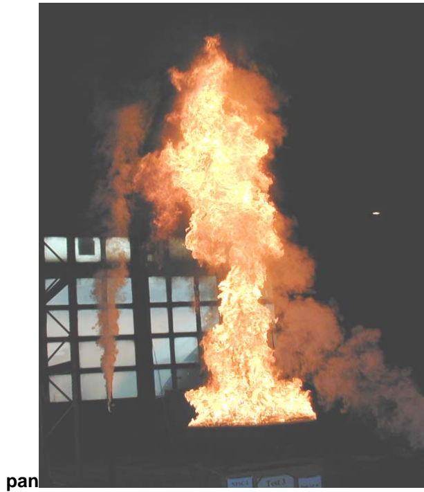
Figure 2-8: Photo of a 2 MW heptane fire during the BE #2 tests. Photo provided by Simo Hostikka, VTT
