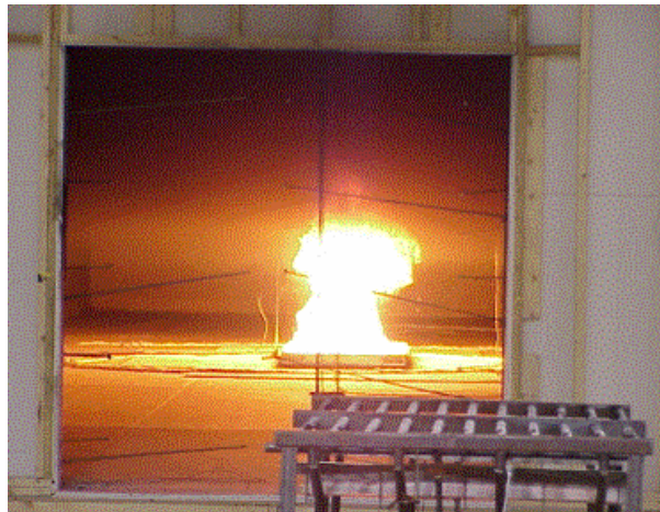
Figure 2-12: Photograph of a 1 MW heptane fire seen through the open doorway. Photo provided by Anthony Hamins, NIST
