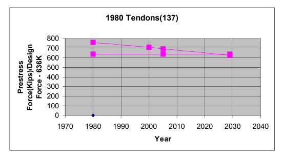
b) Based on the available test information for this set of 23 tendons that were retensioned in 1969, the below graph shows the trend line from 1969 projected through 2005, and out to 2029. The graph also includes a constant line at 636 kips, which is the minimum design prestress force.
