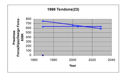
c) Following the initial installation and retensioning of those 23 tendons in 1969, they were then included into the total population of tendons for the structure (160), which were subsequently randomly sampled and tested per Regulatory Guide 1.35 through the year 2000. The next scheduled tendon surveillance will be performed in the year 2005 and will be tested per the requirements of IWL-2520.
