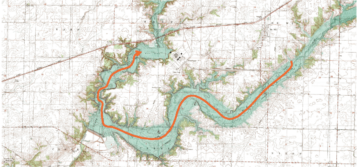
Figure 2.4-2 CPS once-through discharge and subsequent mixing and cooling path
