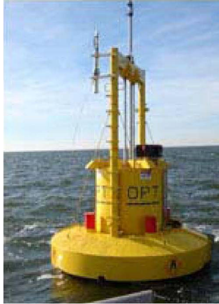
Figure 3-4: An example of a buoy-type wave energy technology.
