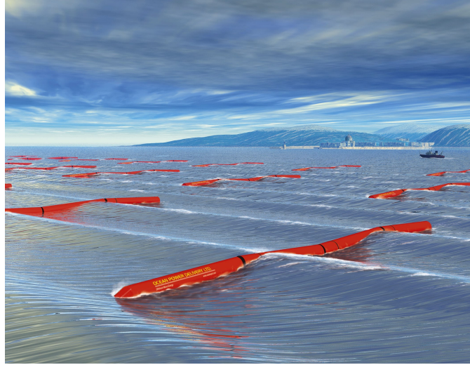
Figure 3-5: Articulated floating cylinders used to collect wave energy.
