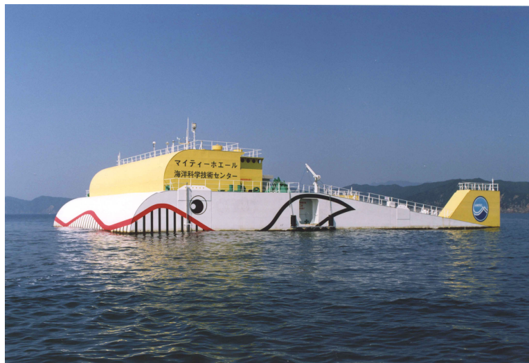
Figure 3-6: Photograph of an oscillating water column device.
