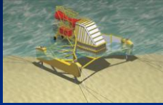
Floating Overtopping Terminator (Wave Dragon)
