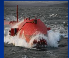
Pelamis 750 kW prototype installed in August of 2004 in 50 m water depth, 2 km offshore the European Marine Energy Centre, Orkney, UK
