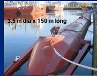
Pelamis 750 kW prototype installed in August of 2004 in 50 m water depth, 2 km offshore the European Marine Energy Centre, Orkney, UK
