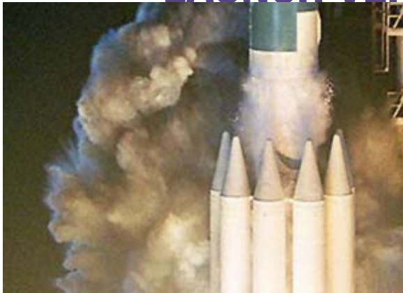
Figure 1: Close-up of the top of the strap-on rocket motors used to increase the main engine thrust.
