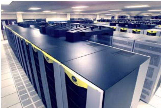
Figure 2: Bird's-eye view of the Columbia supercomputer, a 10,240-processor SGI Altix system comprised of 20 nodes, each containing 512 processors.
