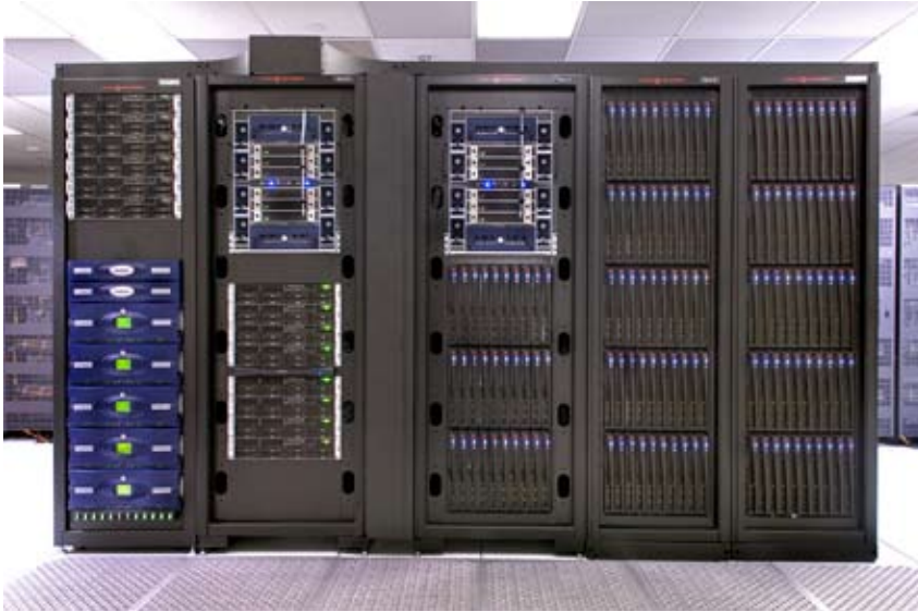
Figure 6: A Linux Network Custom Supersystem called Discover will be the NASA Center for Computational Sciences' next-generation supercomputer. Shown above, the "base unit" of the cluster provides 3.3 teraflops of peak computing power in five closet-sized cabinets.
