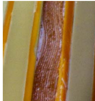
Figure 11. Cable positioning error
