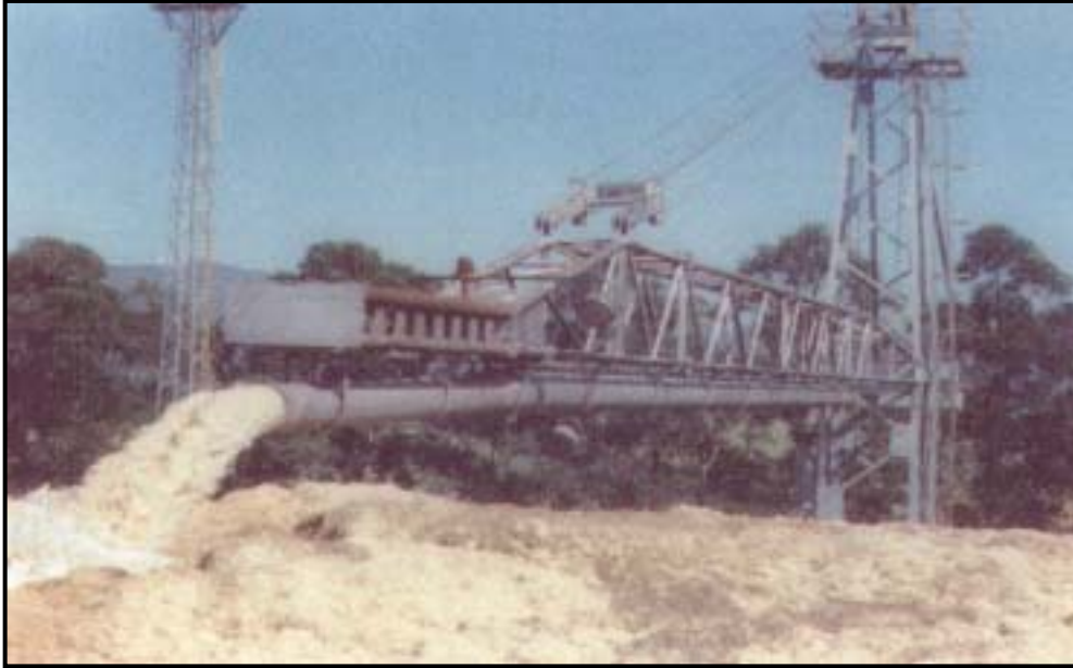
Figure 18 Constructing the Wet Storage Pile: Work Crew Directing the Flow
