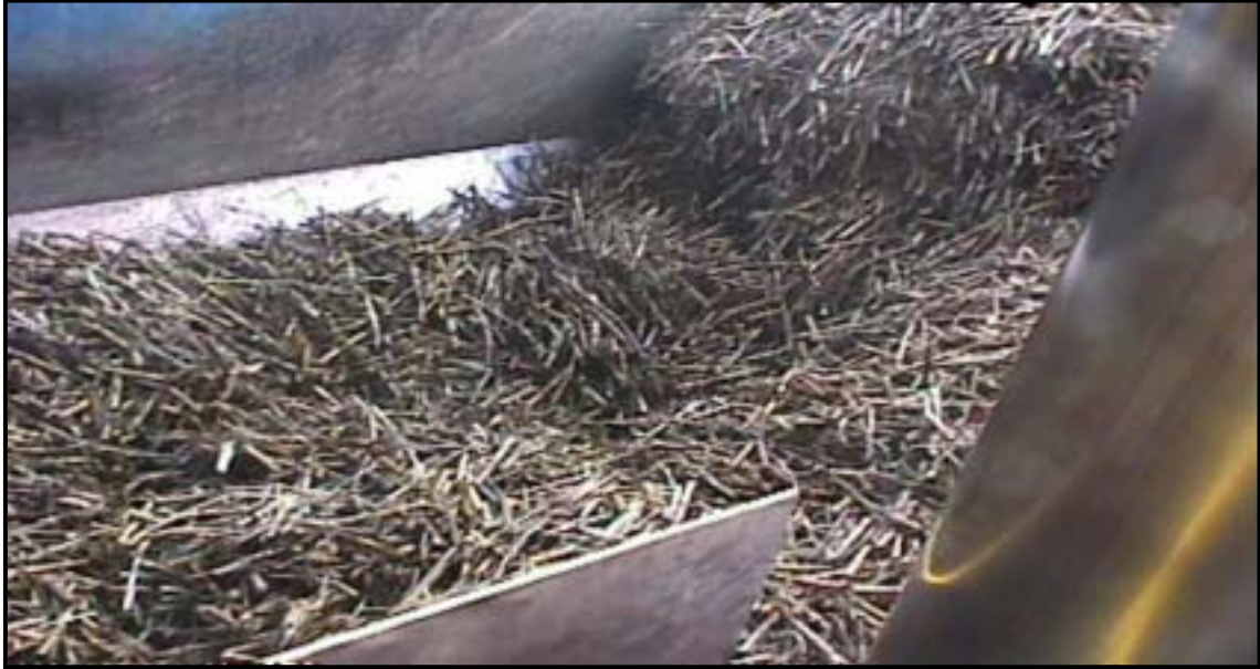
Figure 8 Cane in Conveyor Feed Pit
