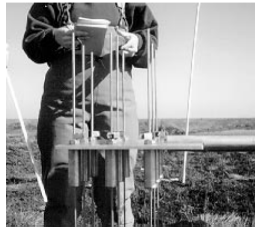
Project monitors shown here use the sediment erosion table technique to measure the accretion (build-up) of sediment in a project area. A flat table is suspended above the marsh surface and nine aluminum rods are inserted through it. Monitors measure the rate of sediment accretion as the distance between the table and the marsh surface decreases. (DNR photos)
