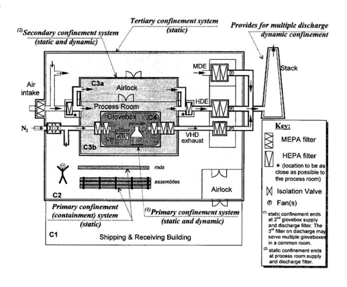
Figure 3-9. Ventilation Confinement for Fuel Fabrication
