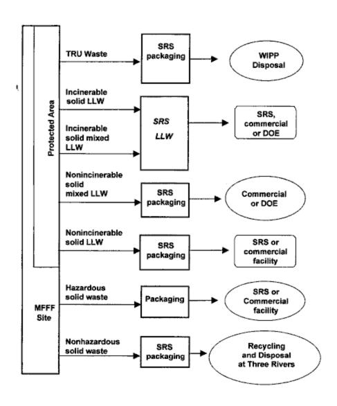
Figure 3-12. Solid Waste Management Flow Diagram
