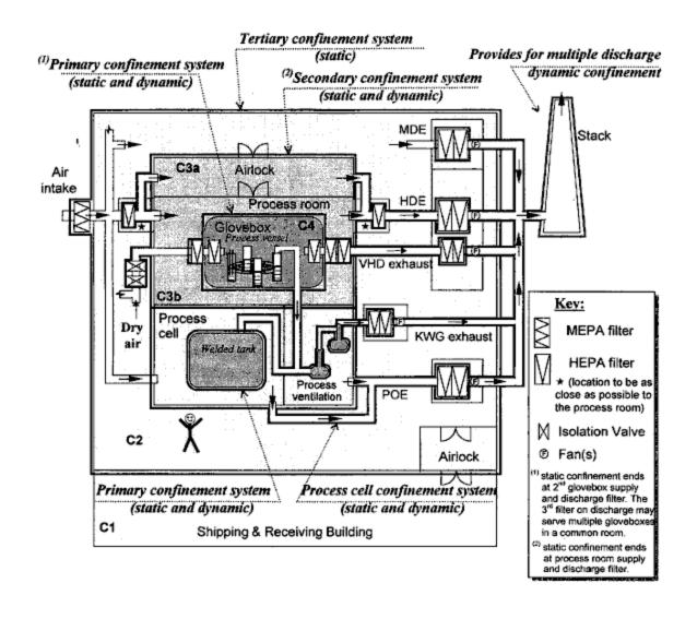
Figure 3-8. Ventilation Confinement for Aqueous Polishing
