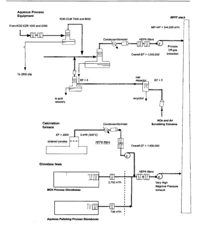
Figure 3-10. MFFF Airborne Waste Treatment Flowsheet
