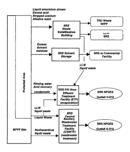
Figure 3-11. MFFF Liquid Waste Management Flow Diagram
