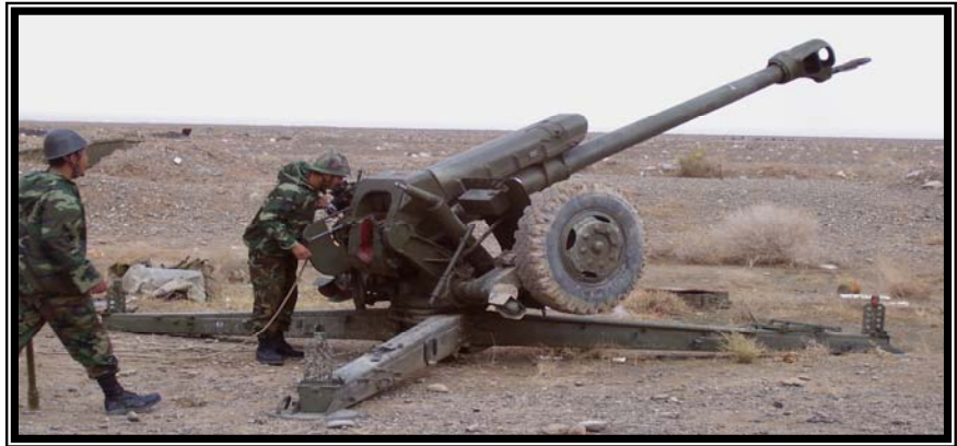
Afghan National Army soldiers assigned to 4th Kandak (battalion), 1st Brigade, 205th Corps prepare a D-30 howitzer gun for firing Nov. 15. The dedicated soldiers are learning to effectively conduct indirect fire using the Soviet-era artillery piece.
