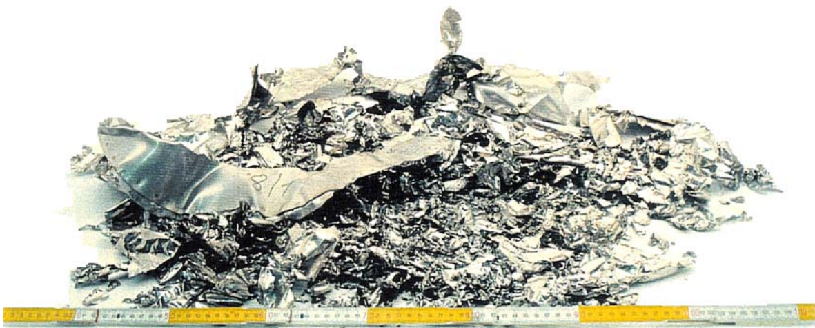
Figure 3-8 RMI Debris Observed in Siemens Steam-Jet Impact Tests
