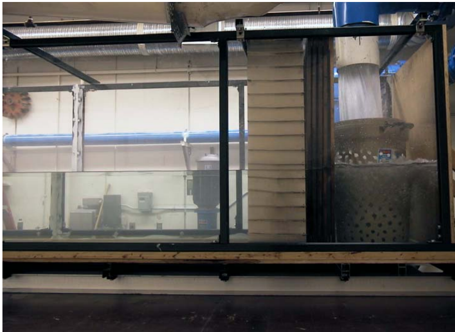
Figure 5-7 Photo of Large UNM Flume Inlet Flow Conditioning Apparatus
