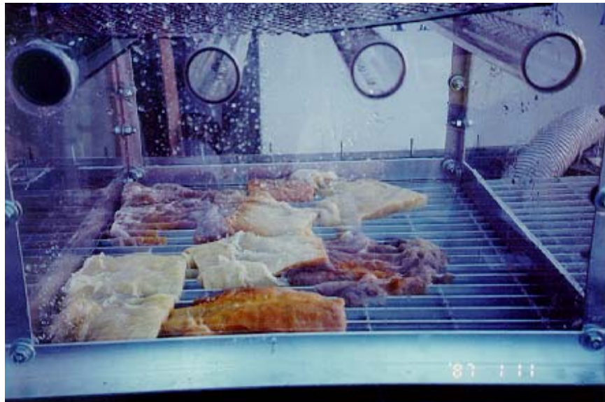
Figure 4-12 Typical Condition of Debris After Exposure to Water
