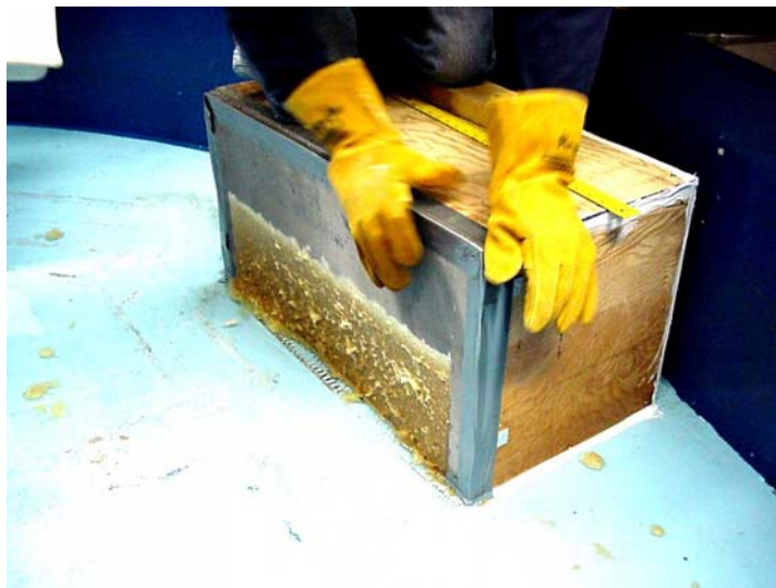
Figure 6-5 Typical Buildup of Fine Fibrous Debris that Easily Remains Suspended
