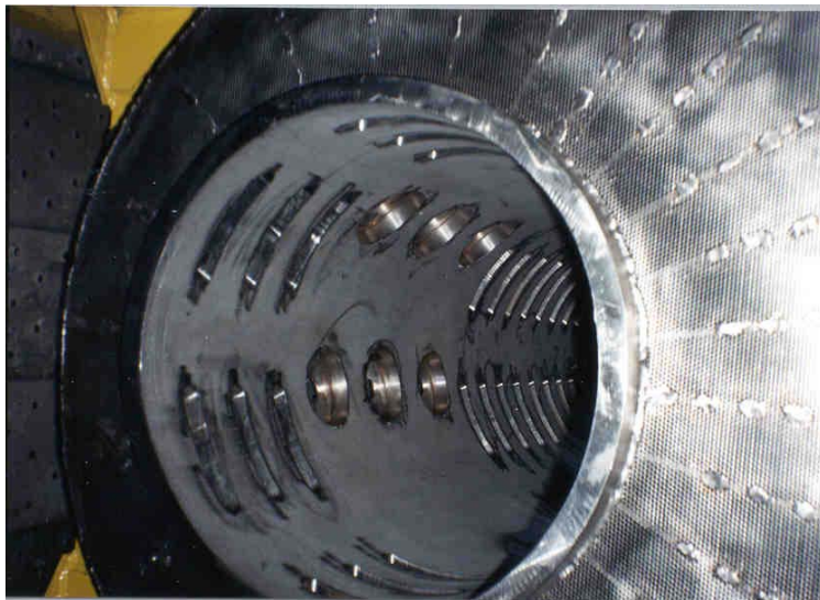
Figure 8-4 The Core Tube Used in the PCI Stacked-Disk Strainers
