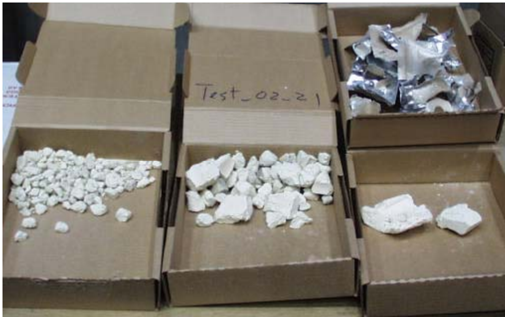
Figure 3-10 Typical Calcium-Silicate Debris Collected from an OPG Two-Phase Jet Test
