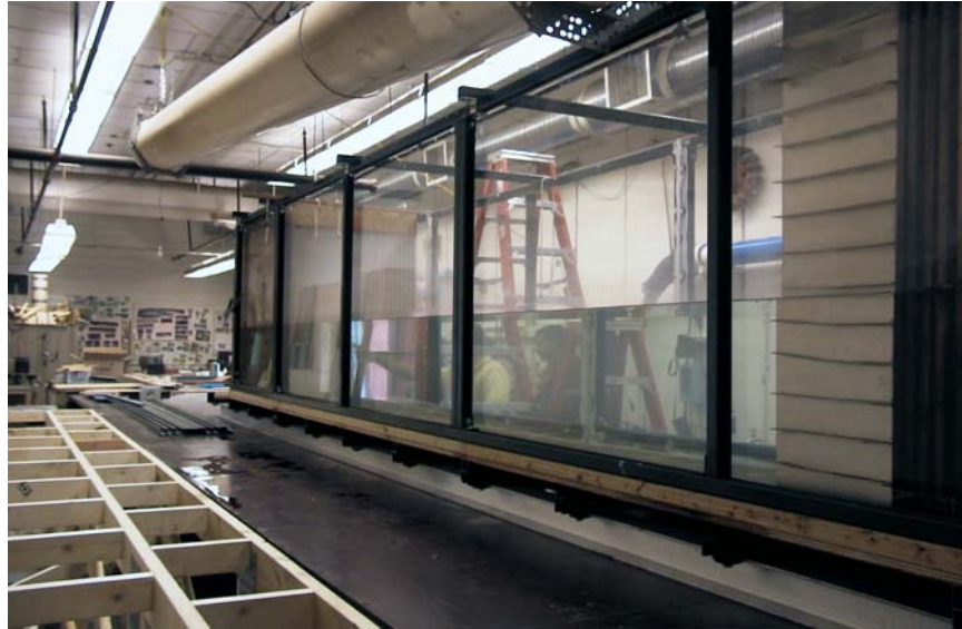
Figure 5-5 Photo of Large UNM Flume Test Apparatus
