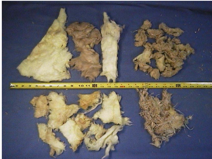
Figure 4-4 Samples of Debris Generated in the CEESI Tests
