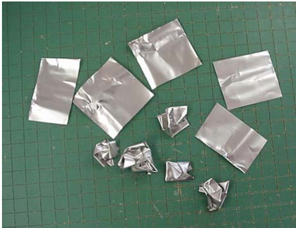
Figure 3-5 RMI Foil Before/After "Crumpling" (Left) and Crumpled RMI Foil Debris (Right)
