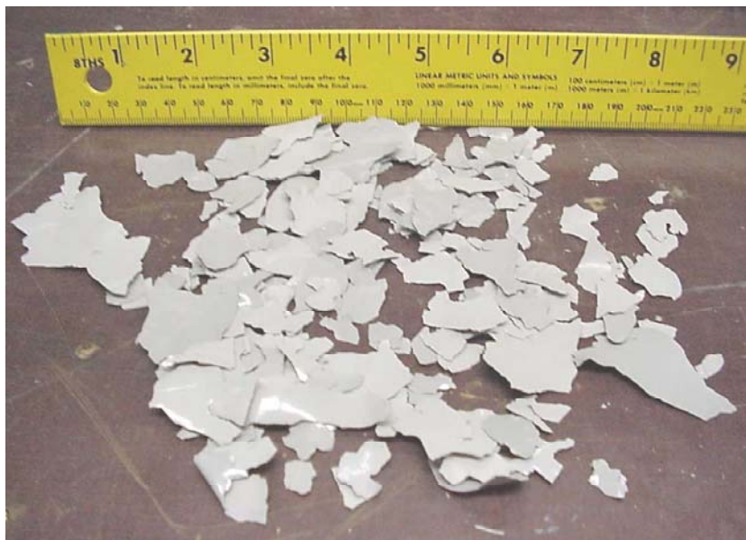
Figure 5-10 Typical Test Sample of Paint-Chip Debris
