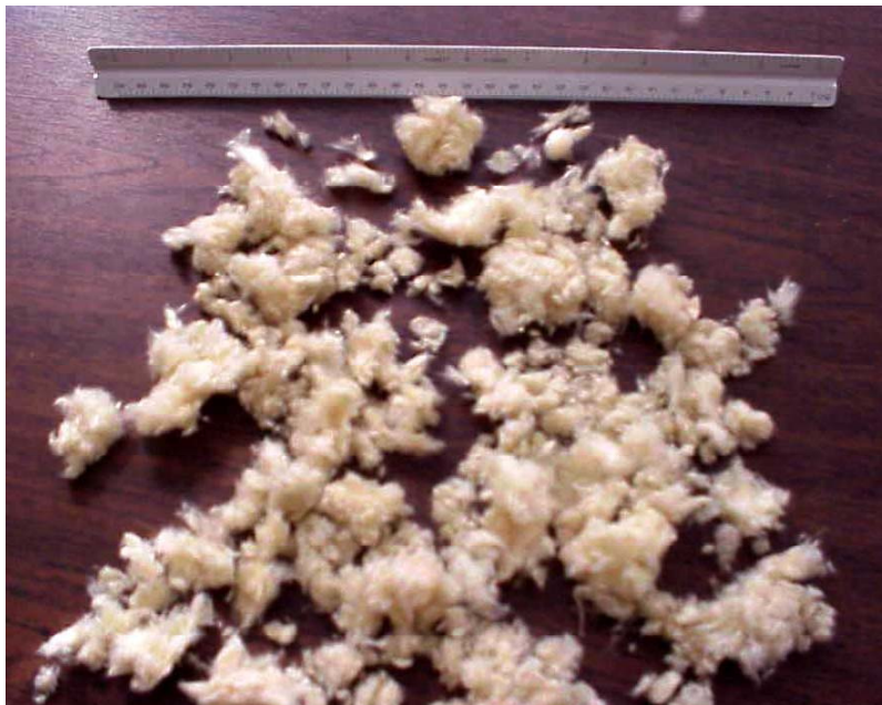
Figure 5-8 Typical Test Sample of LDFG Insulation Debris
