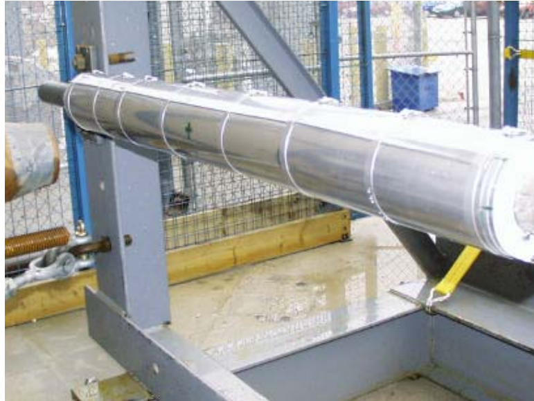
Figure 3-9 Insulation Target Mounting Configuration in OPG Test (Longitudinal Seam at 45°, Circumferential Seam Offset)
