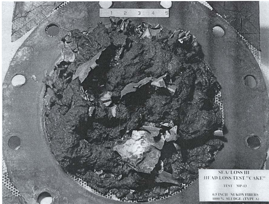
Figure 7-4(a) RMI/Fiber/Sludge Post Head Loss Test Debris Bed
