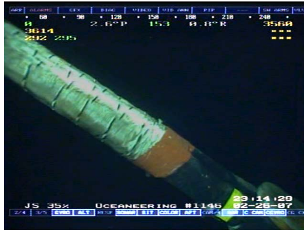
Figure 10. Photograph of Toe of Splice Region
