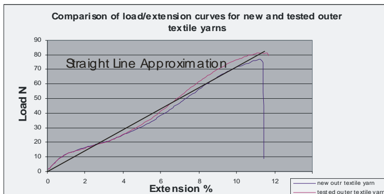
Figure 11 – Straight Line Approximation for Polyester Yarns and Ropes
