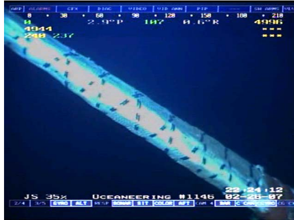
Figure 7. Close-Up View of Rope Condition
