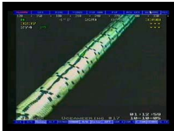
Figure 6. ROV Photograph of Rope Twist
