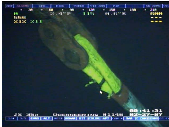
Figure 8. Photograph of Eye Splice and H Link
