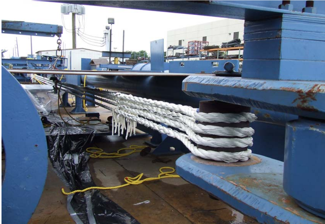
Figure 3. Test Setup for Cycling Four Subropes in Parallel
