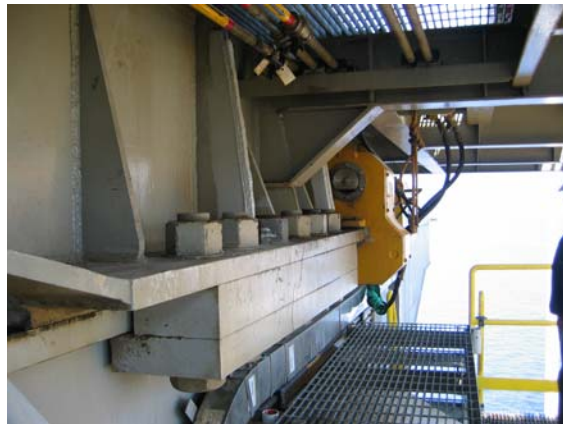
Skid base on deck skid beam - beam on bolted runner guide & hydraulic clamp
