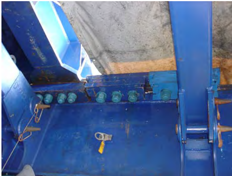
Figure 6 - Reinforced Rig Clamps on Front Runner
