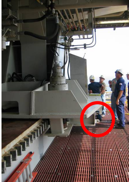
Rack & pinion system to move skid base across deck
