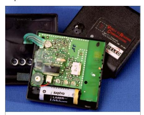
The Delco Type II+ transponder circuitry runs on a Sanyo lithium battery. When the transponder stops working, it probably just needs a new battery. But it will only work with a Sanyo Model CR17450E-R battery. A Salem-based Truck Transponder Service Center specializes in installing new batteries so the transponder can be used for 5-7 more years.
