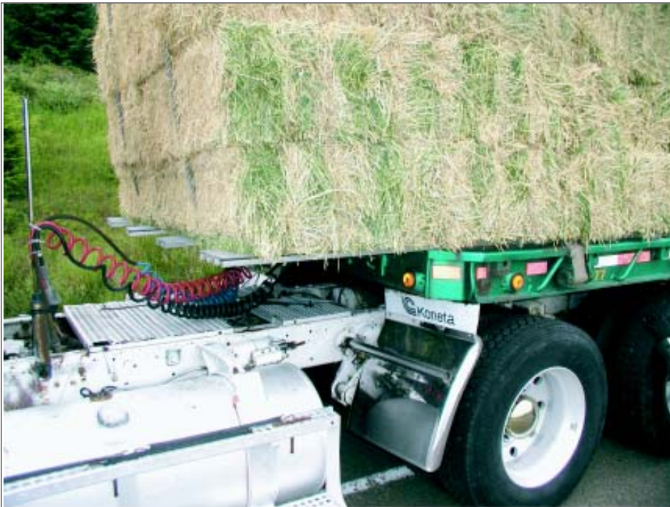
This lead trailer has hay on wood slats that extend forward and add about 4 feet of cargo-carrying capacity, but in Oregon the total combined trailer distance cannot go beyond 68 feet. The maximum length limit has been set in law since the long combination vehicle freeze of 1991.
