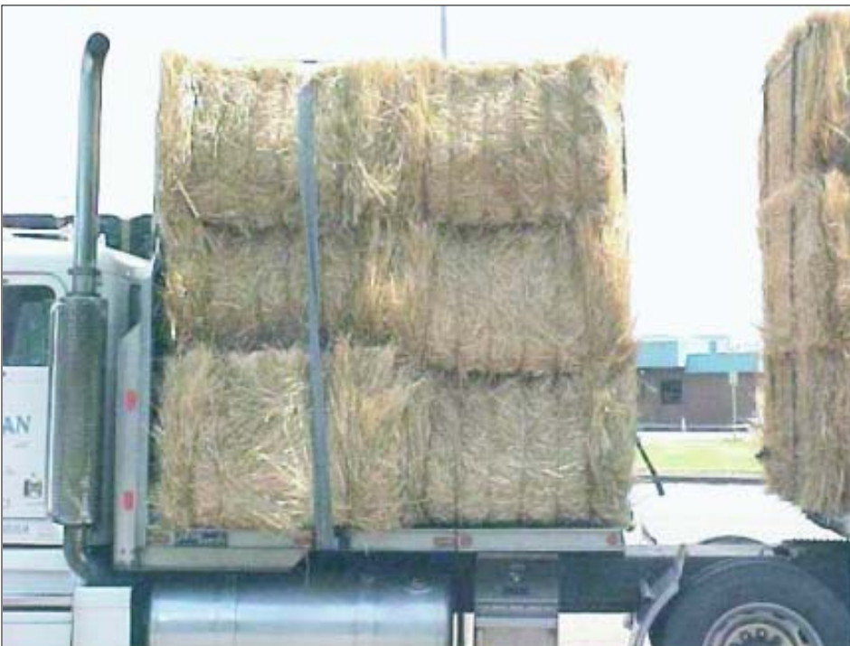
Generally, Oregon laws regarding vehicle length limits allow carriers to use a dromedary truck-tractor to extend cargo-carrying capacity. A truck-tractor with a drom box up to 12 feet 6 inches in length (including the load) may tow a semitrailer and trailer. When the drom box exceeds 12 feet 6 inches, or when the power unit is stinger steered, only one trailer may be towed.
