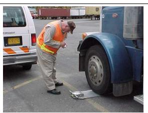
An Oregon motor carrier enforcement officer uses portable scales to check a truck's weight.
