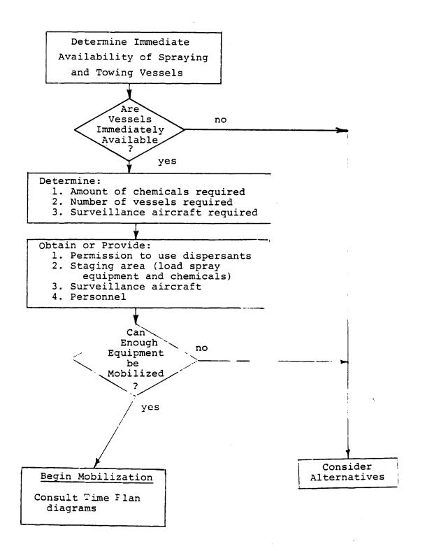
FIGURE 4.11 VESSEL APPLIED DISPERSANT SYSTEM CONSIDERATIONS
