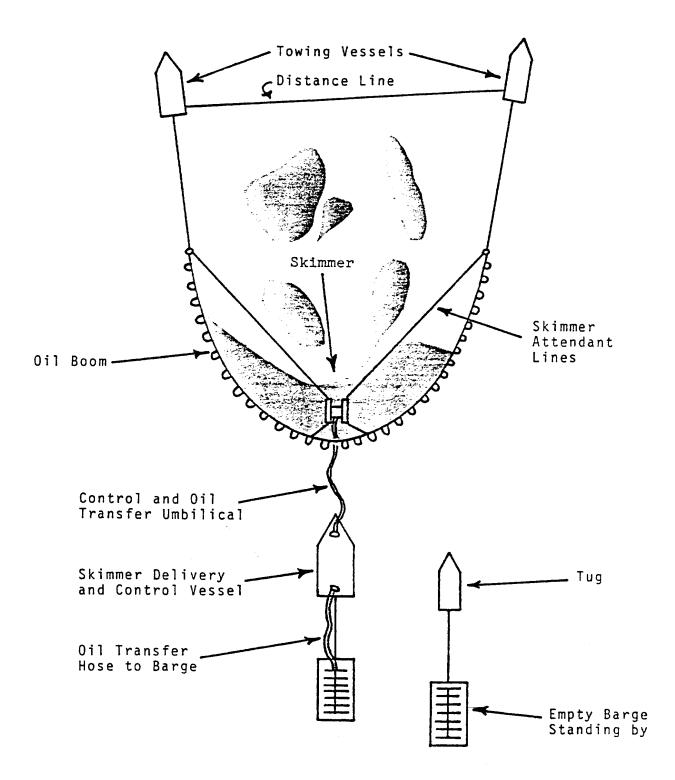
FIGURE 4.5 INDEPENDENT SKIMMER AND BARRIER WITH DISTANT SHIP SUPPORT - FULLY DEPLOYED
