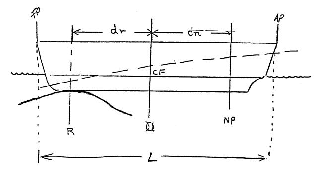
In looking over the above sketch we can see that if weight is added at R, R increases by the amount equal to the weight. As the weight is shifted aft and closer to the neutral point the less effect the weight has on R. If the shift continues past NP going aft it will result in a decrease of R.
