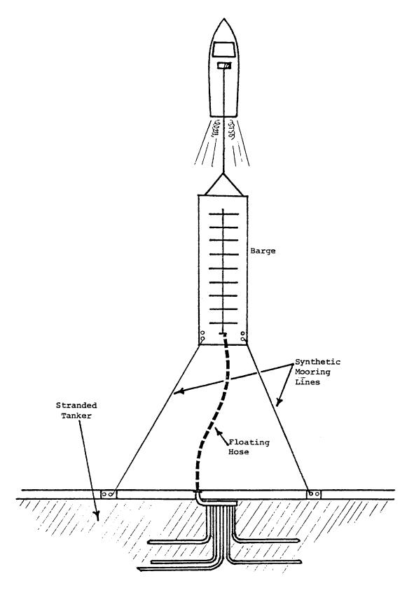
FIGURE 3.3 MOORING SYSTEM FOR OFF-LOADING STRANDED TANKER IN HIGHER SEA STATES
