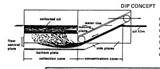
Dynamic Inclined Plane (DIP) Recovery Systems collect oil by forcing it under the surface of the water. Oil follows the surface of the moving inclined plane to a collection well underneath the unit. Buoyant forces cause the oil to naturally separate in the well where it forms a deep oil pocket. Water-free oil is pumped from the top of the well to storage.
