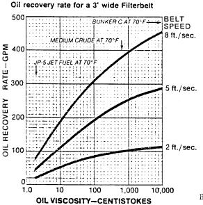
Oil recovery performance is a composite of laboratory and test basin data, confirmed by field experience. Curves are shown for the maximum oil recovery rate (saturation) of the Filterbelt.
