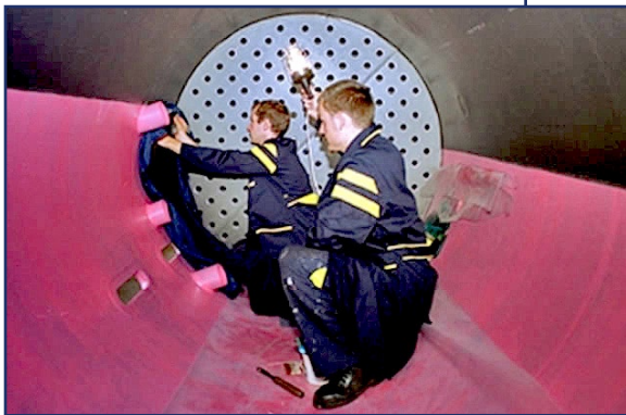
Workers install rubber molding at a Gumiimpex's factory in Varaždin, Croatia.
