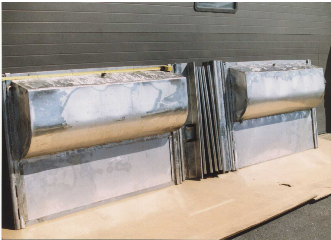
Figure 3-3. Redesigned Pocket Boom as Built by Applied Fabric Technologies.
