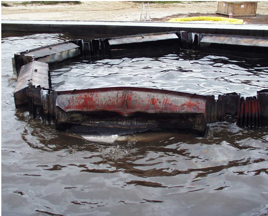
Figure 6-6 View of Flotation Unit After Crumpling Incident at End of Third Burn
