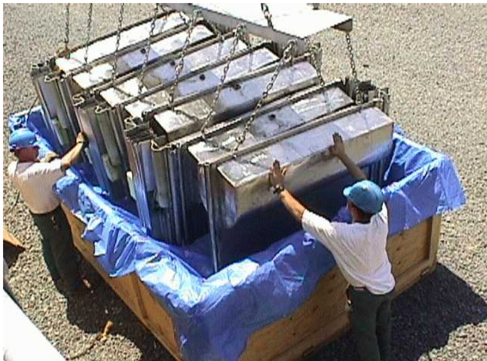
Figure 10-2. Deployment of 15 m (50 ft) of Pre-connected Pocket Boom.
