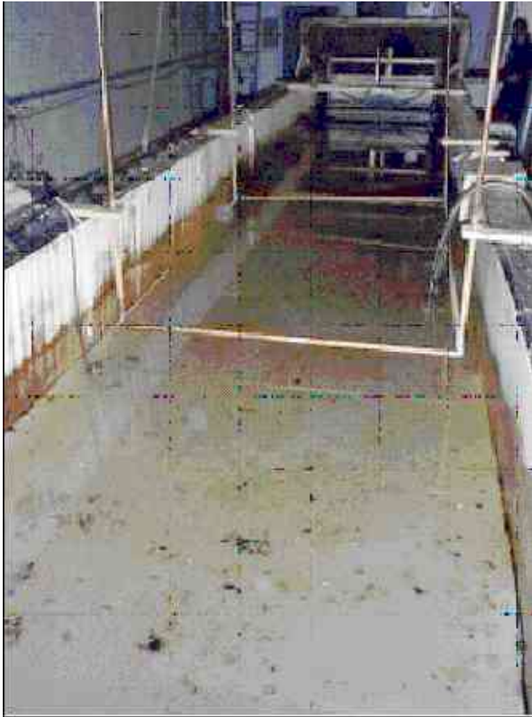
Figure 2: Air Bubble Barrier Piping
