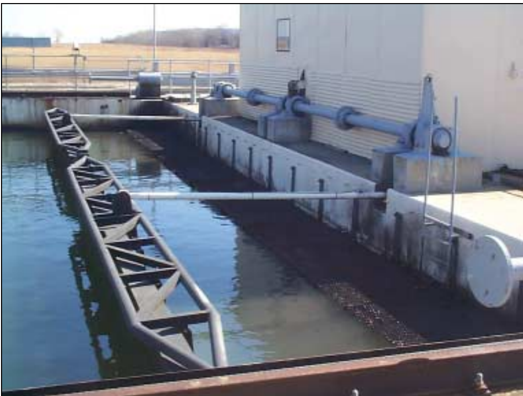
Figure 3. Ohmsett Tank Wave Paddle System
