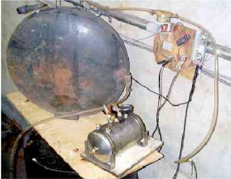
Figure 4. Dispersant Spray Pressure Tanks and Valve
