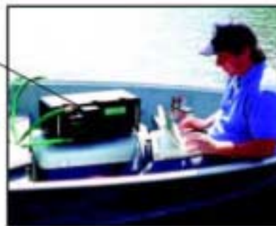
The 10-AU configured with the 25 mm One-Piece Flow Cell, a garden hose, and a 12 VDC cable for continuous field operation.
