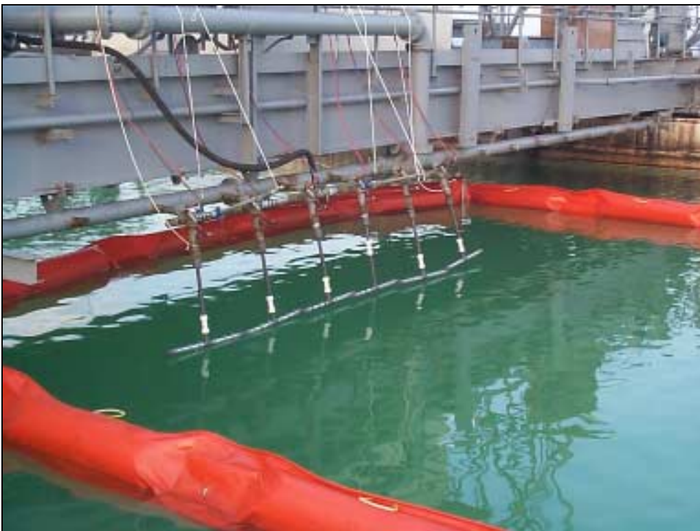
Figure 5. Oil Distribution System
