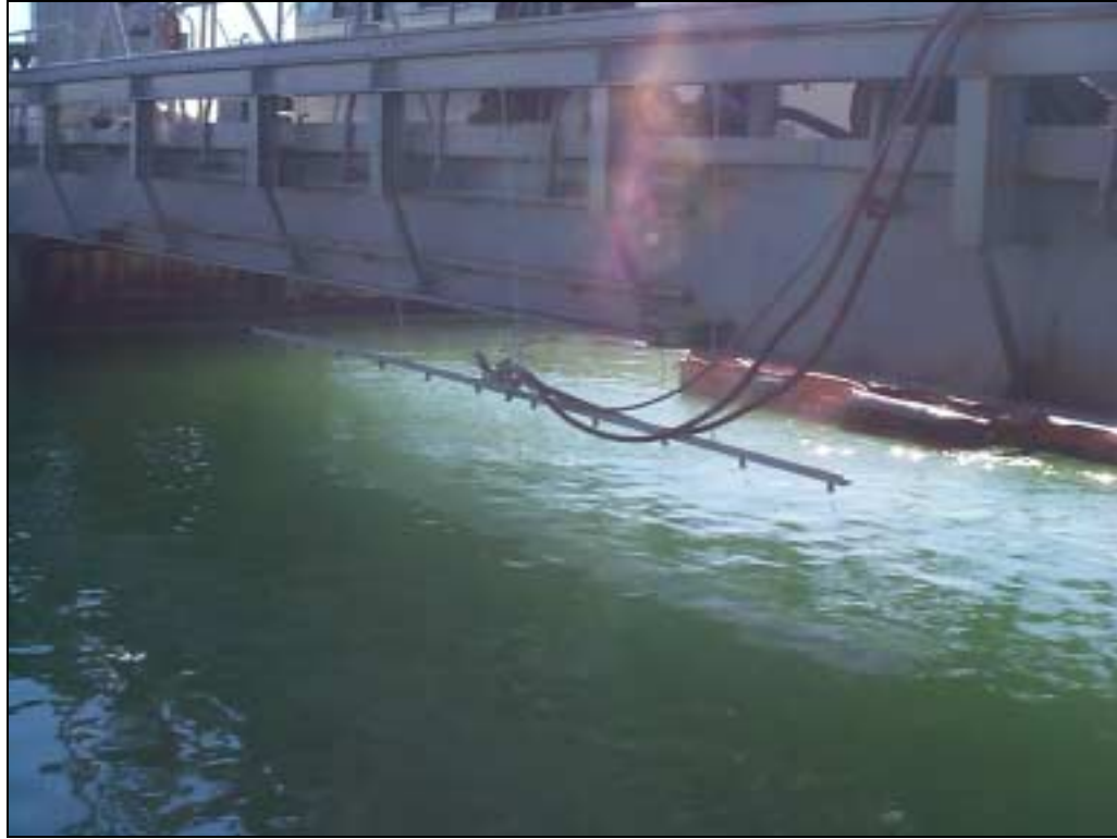
Figure 8. Dispersant Spray Bar in Operation
