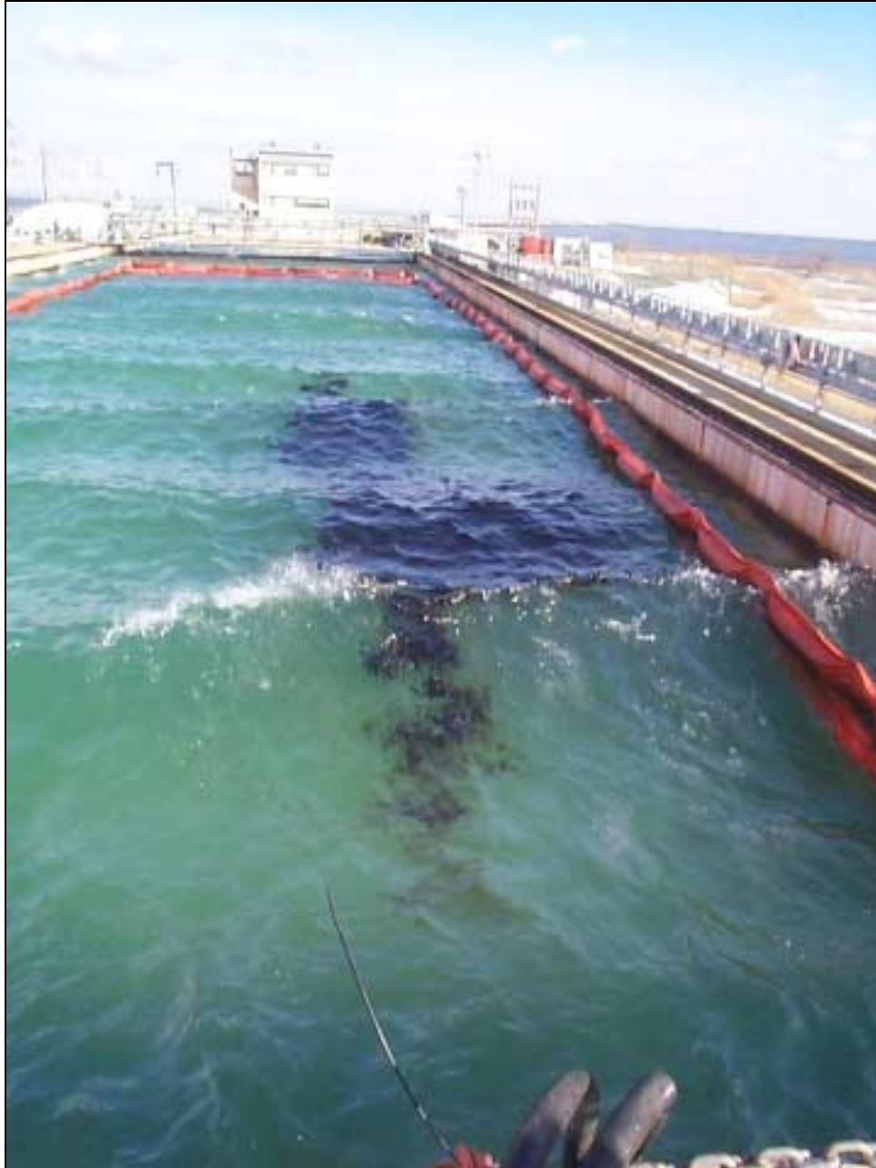
Figure 9. Control Test (no dispersant), Surface Oil an Cresting Wave
