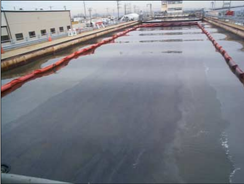
Figure 2. Ohmsett Test Tank with Oil Containment Boom
