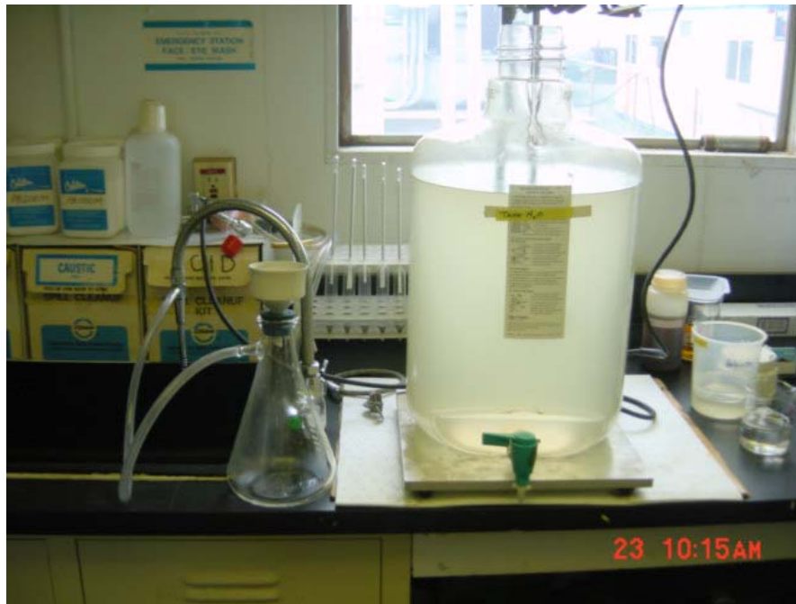
Figure 5: Apparatus for dispersant removal by PAC bench tests.
