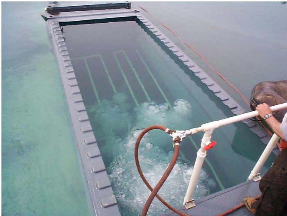
Figure 18: Checking operation of bubbler system.
