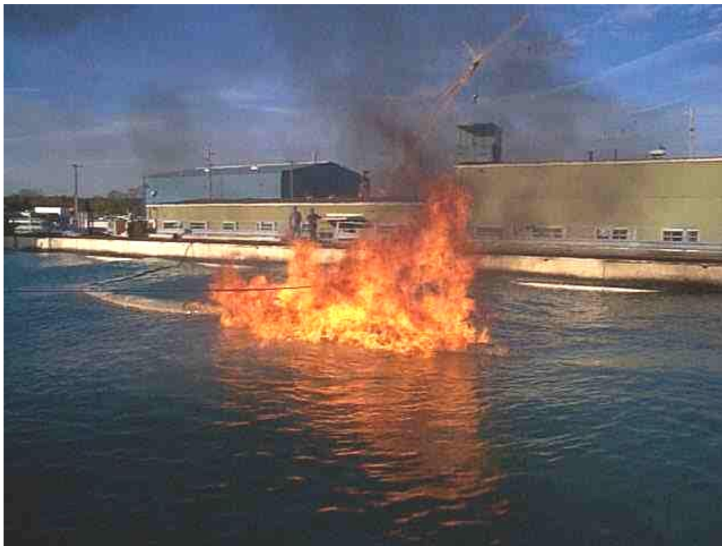
Figure 5. Boom undergoing burn test in waves.
