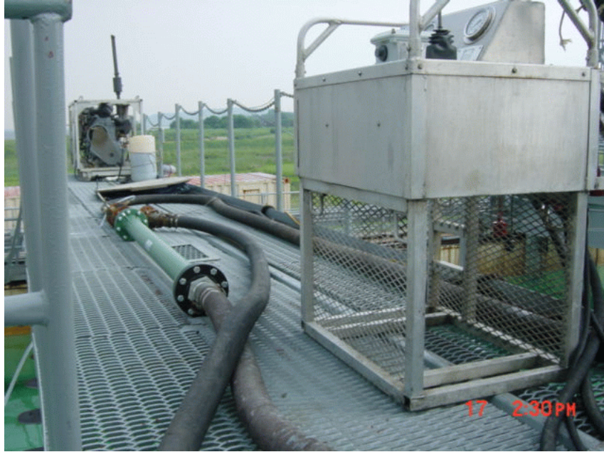
Figure 6-4. In-line mixer on Auxiliary bridge deck.
