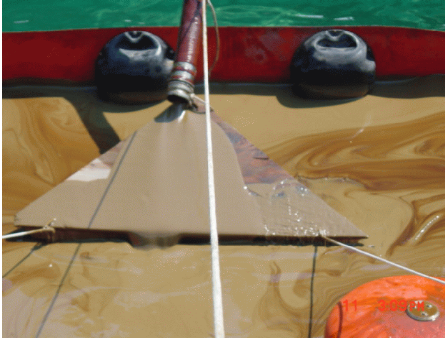
Figure 6-10. Spill plate and distribution of emulsion inside boomed area.
