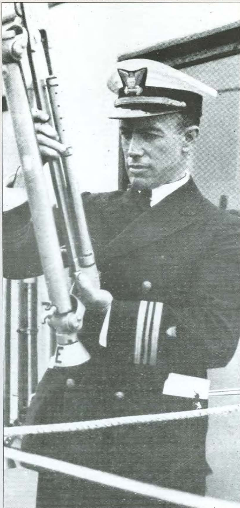
"Iceberg" Smith as a lieutenant commander and leader of the Marion expedition, studies the readings from a Greene-Bigelow water bottle, a device used to sample water quality and temperature.
